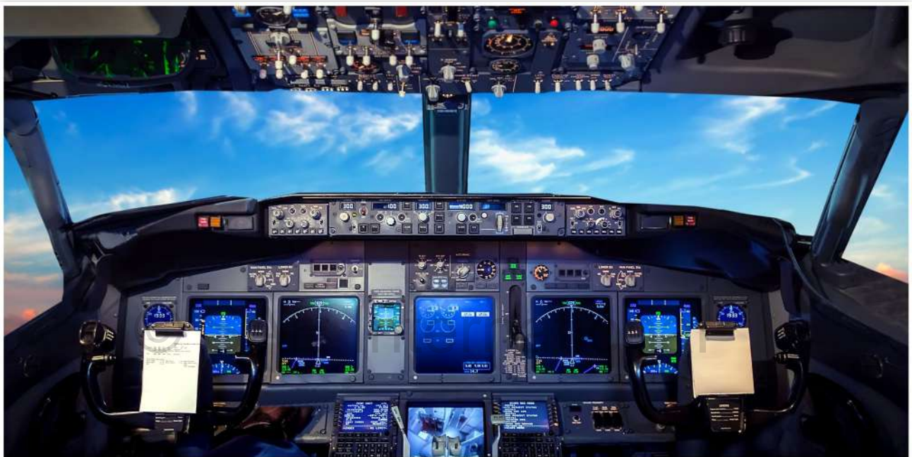
FIGURE 2. Most modern cockpit systems are comprised of avionics that use IMA architectures, such as the Honeywell AIMS system.
