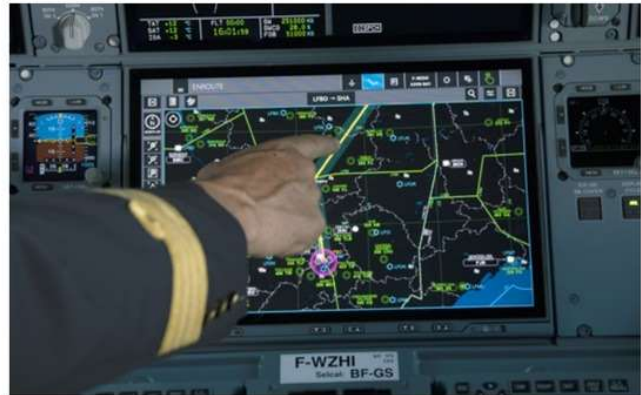
Standards cover aircraft from stem to stern, including electronics. Shown is the Airbus A350 XWB cockpit touchscreen.
